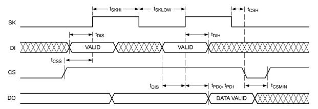
Figure 2. Synchronous Data Timing
